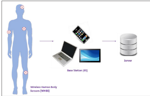
Figure 1: Architecture of wireless human body sensors in healthcare applications.
