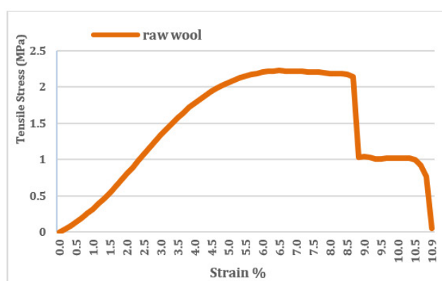
Figure 9: Stress -strain curve of dyed wool yarn and raw wool yarn.
