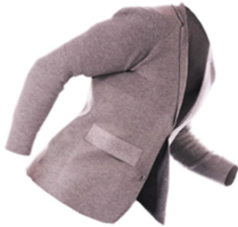
Figure 7: 3D printed jacket without seams.
