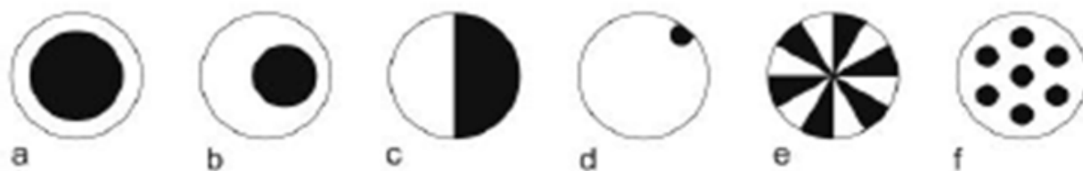
Figure 3: a) centric center-shell (C/S), b) eccentric center-shell (C/S), c) equal side-by-side (S/S), d) unequal side-by-side (S/S), e) sliced cake, f) islands in the sea (I/S) as spinneret profiles of Bi-Component spinning technology (BCY) [5].
