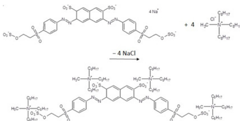
Figure 1: Ion exchange reaction of Novacron Black NN reactive dye and commercially available ionic liquid Aliquat 336 produces insoluble ion pair.
