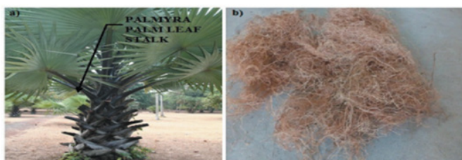
Figure 1: (a) Palmyra Palm Leaf Stalk (b) Extracted Palmyra Palm Leaf Stalk Fiber [9].
