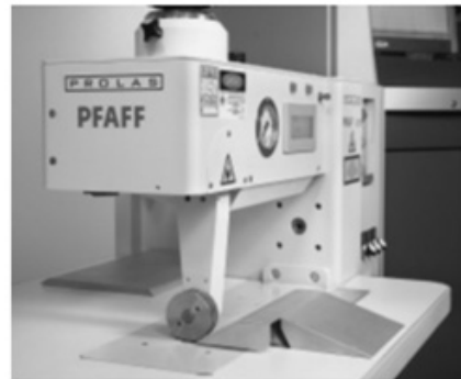
Laser welding machine
