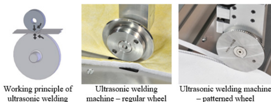
Figure 3: Ultrasonic welding working principle and commercial welding machines [9,11].
