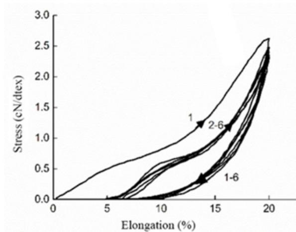
**Figure 3:** Elastic recovery of elastomeric yarn for the initial elongation at 20%.
