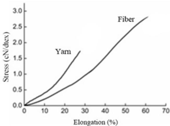
**Figure 2:** Typical Stress-strain curves of elastomeric fiber and yarns.
