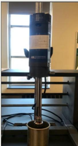
**Figure 4:** The Nano mixer used to make the printing ink.
