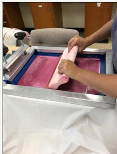
**Figure 7:** The fabric printed with squeegee using the prepared screen.
