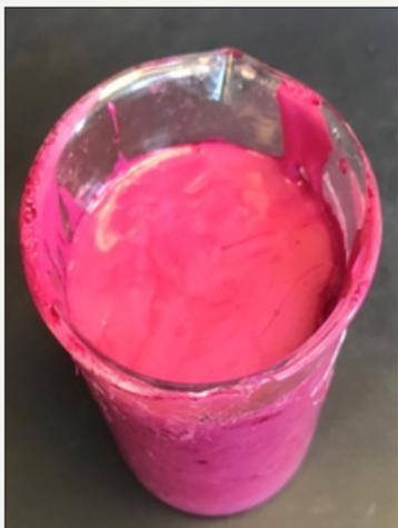
**Figure 5:** The ready printing ink using cochineal pigment and the thickener.
