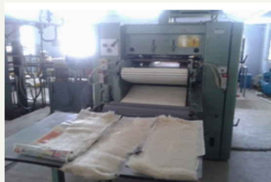
Figure 3: Needle punching of silk and wool fiber web.
