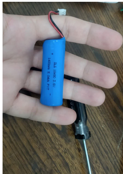
Figure 2: Lithium battery of light cure device.
