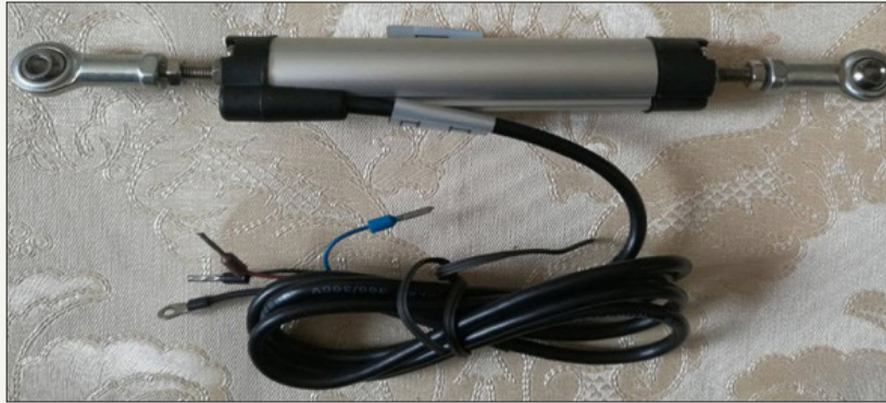
Figure 4: WYJ-V-150 mm displacement-sensors linear sensors.
