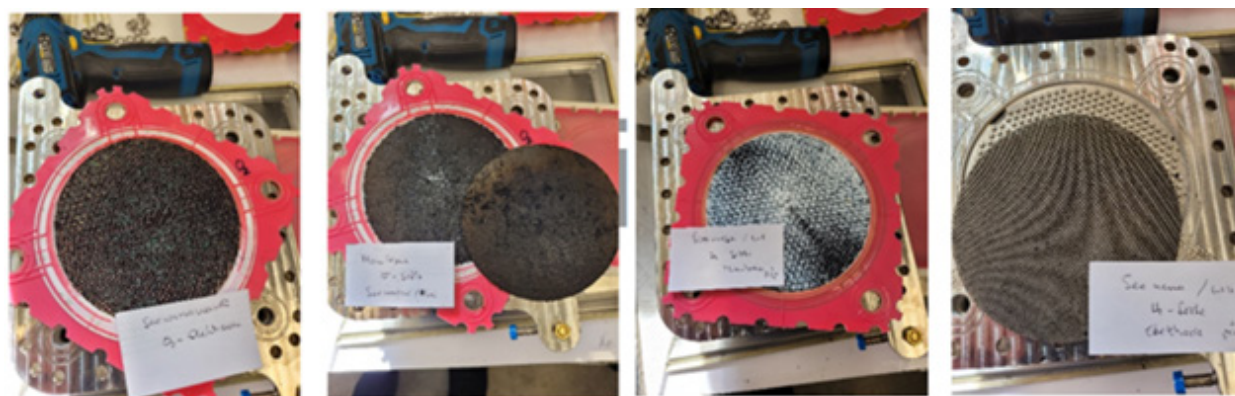
Figure 5: Post-mortem appearance: O 2 -side (A/B) & H 2 -side (c/D) electrodes after seawater electrolysis.
