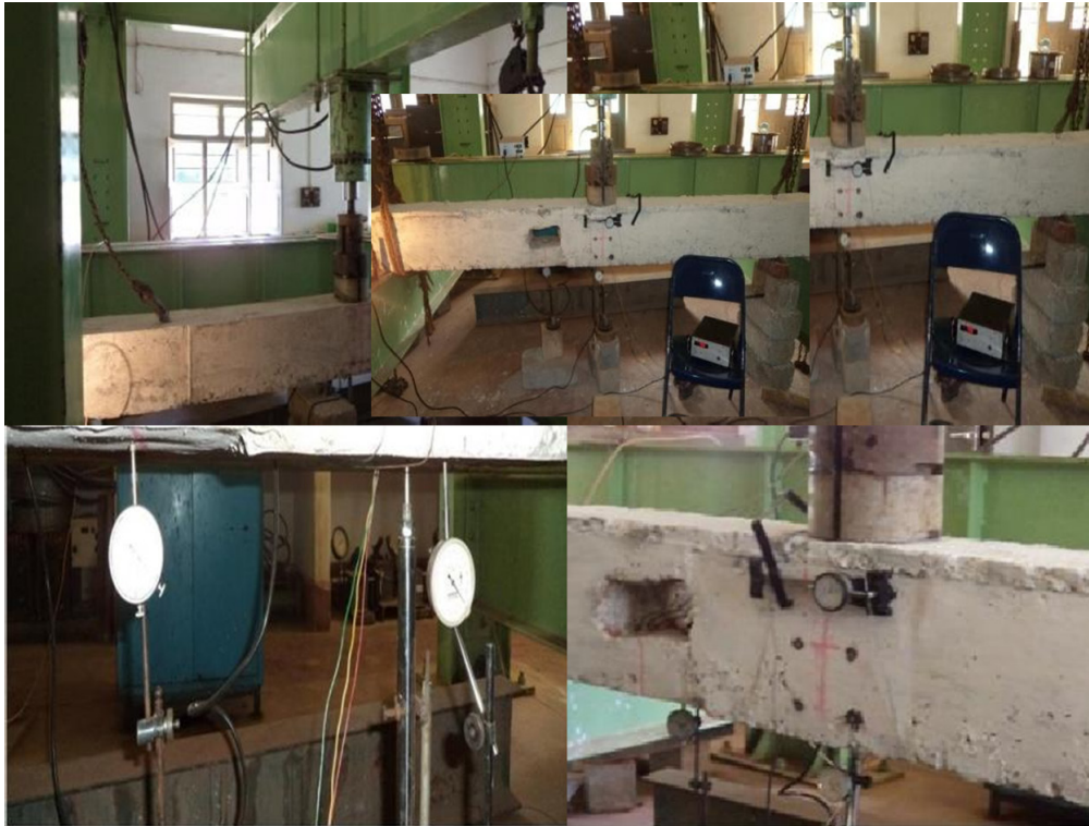
Figure 2: Clockwise: beam, with cutout, dial gauge and sensor and Demec gauge arrangements.
