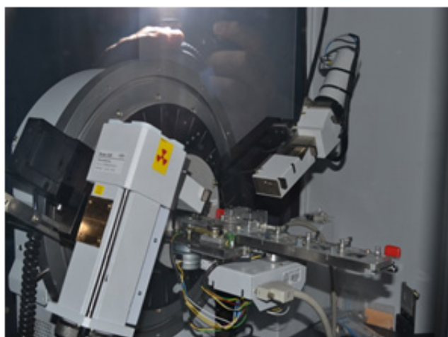
Figure 4: Bruker D8 ADVANCE X-ray diffractometer. Diffraction cell showing the X-ray monochromator (left) and the detector collecting the sample's reflection (right).
