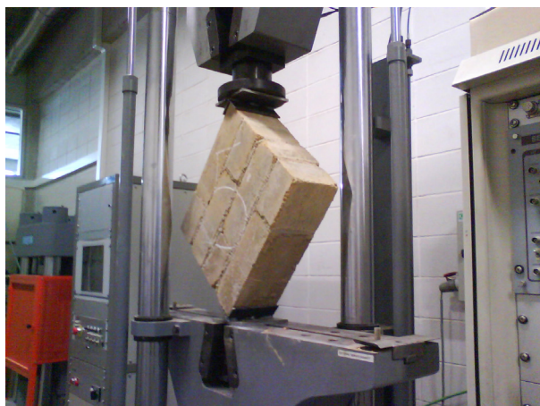
Figure 8: Earth block shear test conducted at Girona University Laboratory [17].
