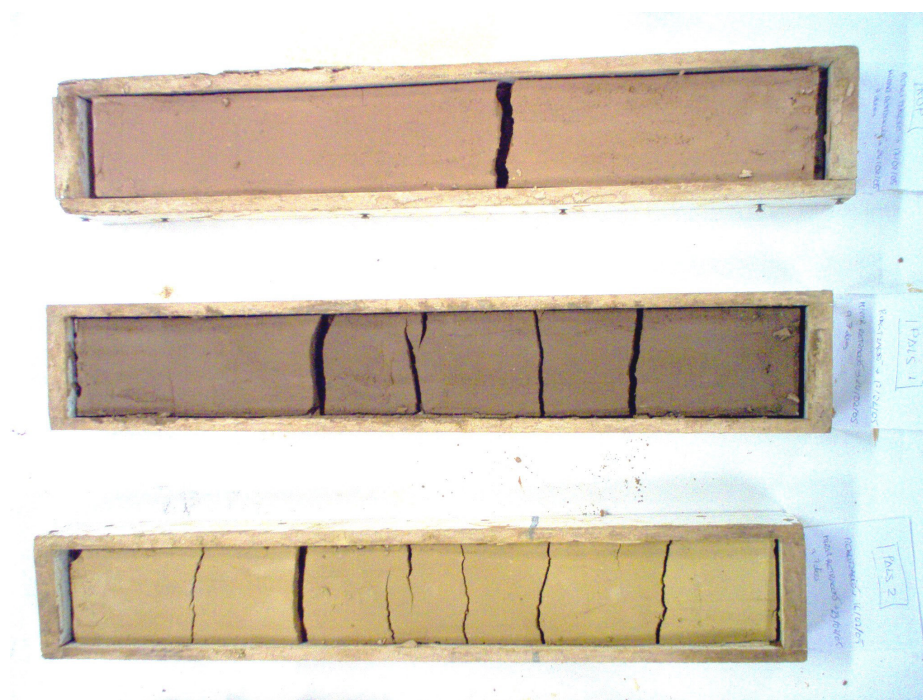
Figure 6: Shrinkage test on three soil samples for rammed earth.
