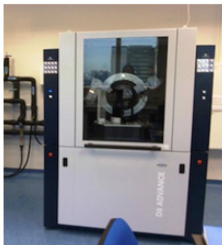
Figure 4: Bruker D8 ADVANCE X-ray diffractometer. Diffraction cell showing the X-ray monochromator (left) and the detector collecting the sample's reflection (right).
