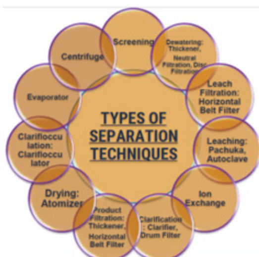
Figure 10: Types of separation techniques in mineral processing plant.
