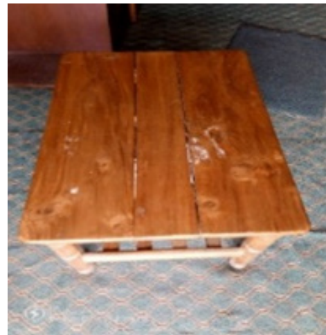
Figure 6: Delaminated table top.
