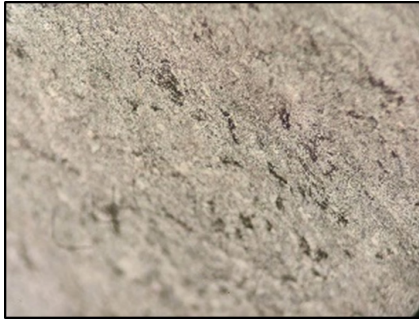
Figure 6: Microstructure of the cast lead rod.
