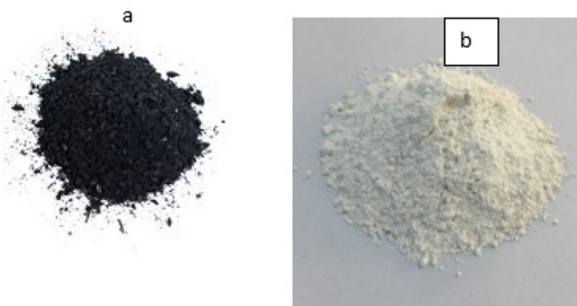
Figure 2: (a) Treated POFA furnace for 1.5h at 600 °C (b) Prepared porcelain powder.
