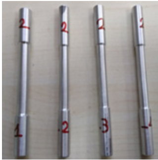
Figure 3: Machined round tensile test bar specimens form hot swaging operation and heat treated for T6 condition. The tensile test results are given in Table 1.
