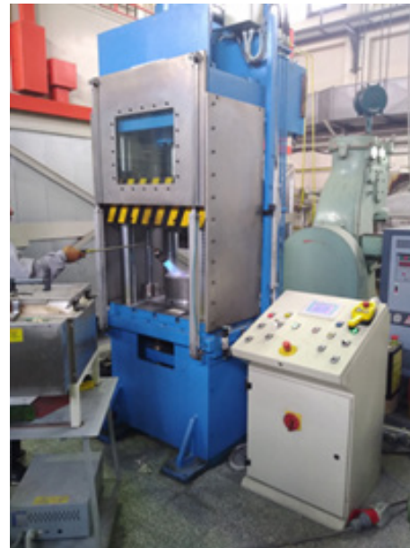
Figure 1: Automated 100 Ton hydraulic press used for hot forging experiments at METU.
