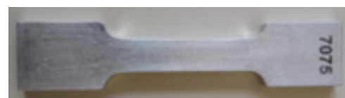
Figure 2: First group AA7075 consist of hot forged slabs machined into flat tensile test specimens.
