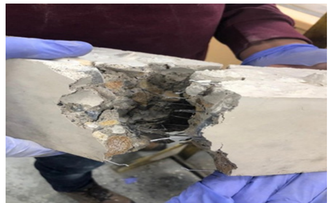
Figure 33: SF2 Prism after crack.
