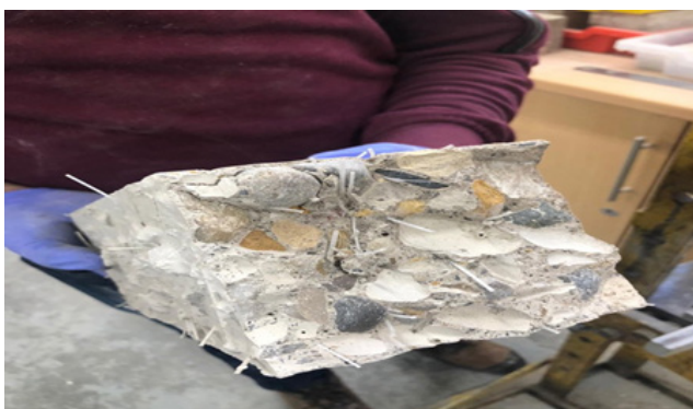
Figure 27: PPF2 Prism following failure.
