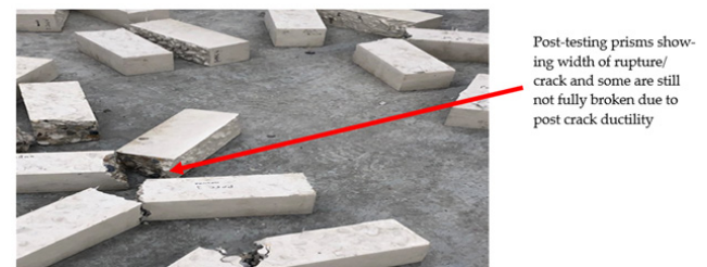
Figure 17: Prisms after crack.
