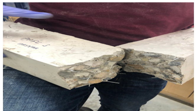
Figure 25: PPF1 Prism after rupture.
