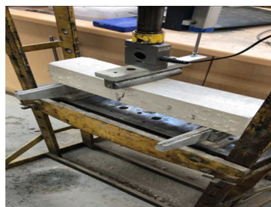
Figure 11: Prism testing for flexural strength.
