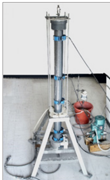
Figure 1: Laboratory equipment for penetrability evaluation [9-15].
