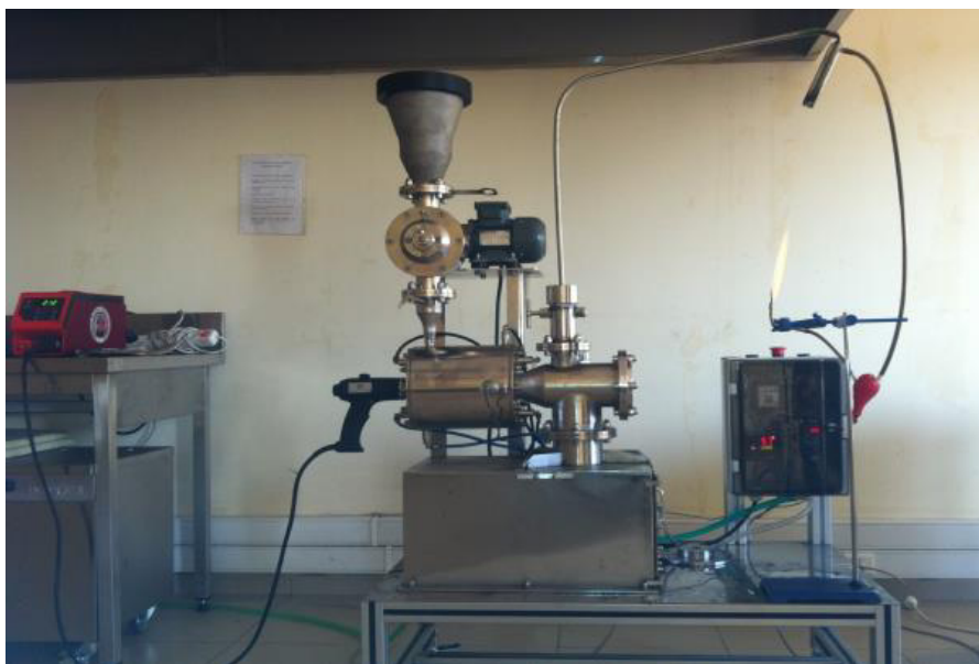
Figure 2: Experiment setup with integrated arc plasma system.
