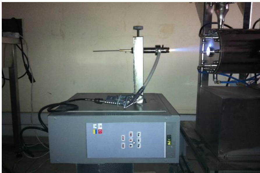
Figure 3: Experiment setup with integrated microwave plasma system.
