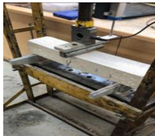
Figure 3: Flexural testing of prisms.
