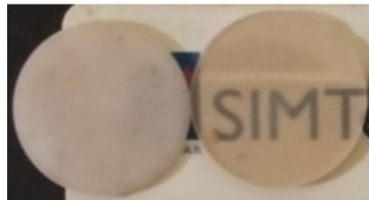
Figure 4: As sintered yttria discs a) without and b) with zirconia additive.
