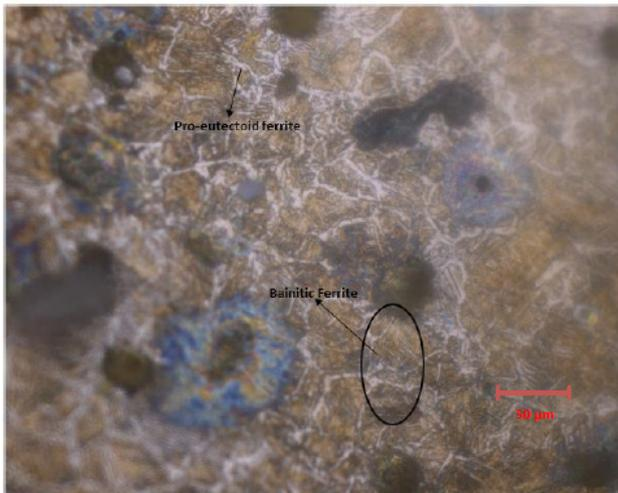
**Figure 4a:** Microstructure of step up austenitized ADI (Batch A).
