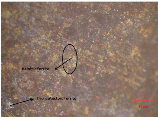
**Figure 4b:** Microstructure of step austenitized ADI (Batch B).
