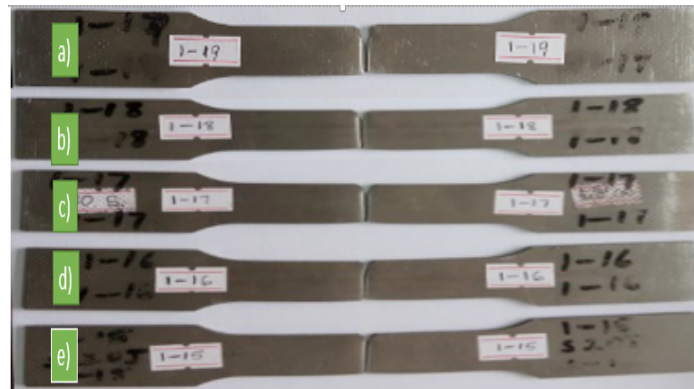
Figure 7: Images of material with and without LSP after fracture: a) NOLSP, b) S20J, c) S30J, d) D20J and e) D30J.
