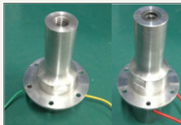
Figure 10: Ultrasonic amplitude transformer (a) 28000Hz amplitude pole (b) 14000Hz horn.
