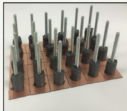
Figure 4: Solder bump tensile testing samples.
