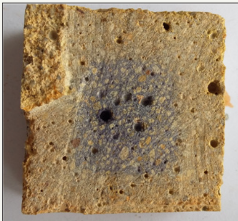
Figure 1 : Example of the carbonation front measured by using the blue timol indicator solution. The easiest and most widely carbonation model used in mortars and concretes is shown in Eq. (1).
