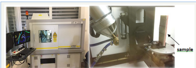
Figure 4: The NIKON XT H 225 CT system and the damaged sample.
