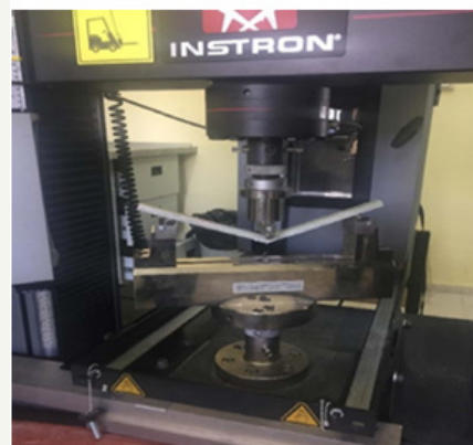
Figure 3: 3-Point Bending test for the composite specimen.
