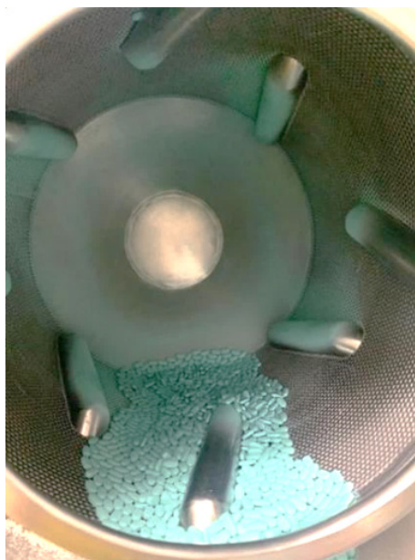
Figure 6: Illustrative photo of the internal part of the coating machine in the manufacturing of Valeriana officinalis L. 50mg tablets.
