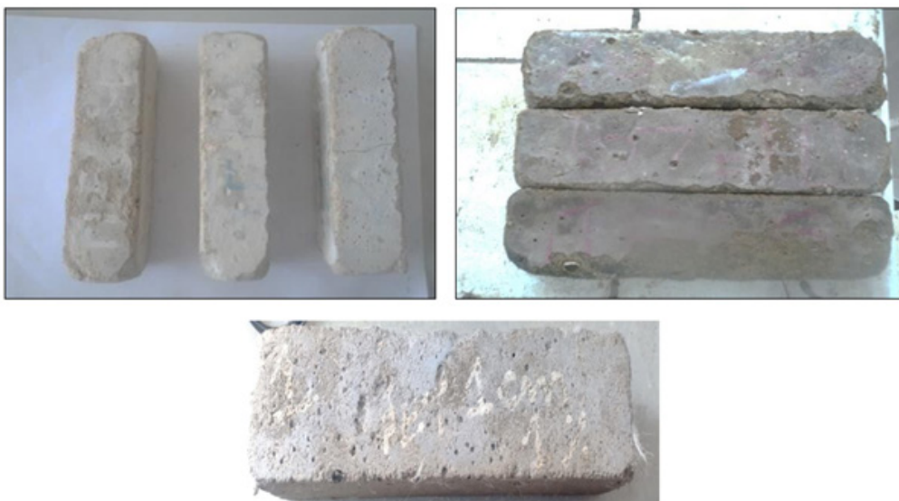
Figure 7: Visual observation of mortars exposed to magnesium sulphate solution.
