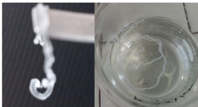
Figure 3: Regenerated material after the wet spinning process.
