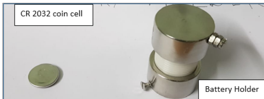
Figure 1: Photograph of the fabricated coin cell and the battery holder.
