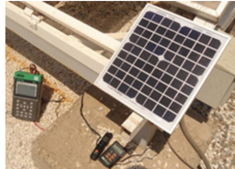
Figure 12: The solar panel, radiation meter, thermometer and solar panel test device.
