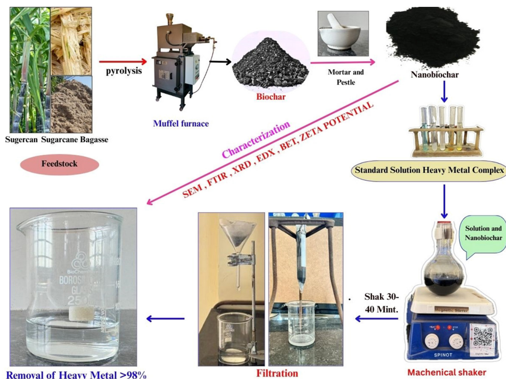
Figure 1: Preparation, characterization, and application of sugarcane bagasse-derived nanobiochar for heavy metal removal (>98%).
