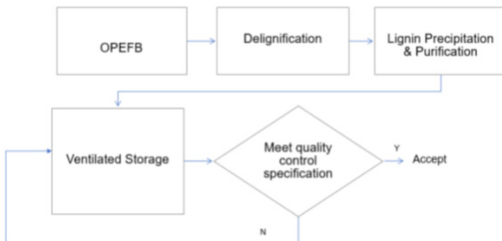
Figure 1: Lignin pretreatment from OPEFB into high purity product.
