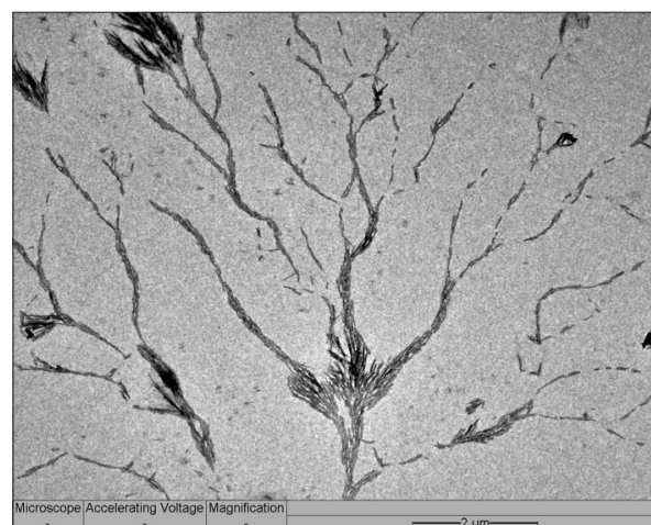
Figure 6: The tree-like growth on the AC flakes prepared by the microwave-aided deposition approach.
