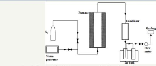
Figure 1: Schematic diagram of a fixed bed reactor system used in this study.
