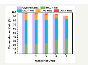
**Figure 5:** Reusability of 20% (w/w)  $SO_4/K10$  catalyst for acetylation of glycerol at molar ratio of 1:12 (glycerol: acetic acid), catalyst loading of 0.4g, 120 °C and 5h.
