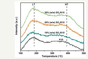
Figure 2: NH<sub>2</sub>-TPD profiles of parent K10 and Sulfonated K10 catalysts.
