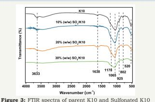
Figure 3: FTIR spectra of parent K10 and Sulfonated K10 catalysts.
