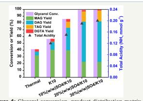
Figure 4: Glycerol conversion, product distribution matrix along with the total acidity of K10 and Sulfonated K10 catalysts at reaction conditions: molar ratio of 1:12 (glycerol: acetic acid), catalyst loading of 0.4g, 120 °C and 5h.
