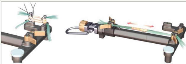
Figure 1: Preparation and fixation of the ST4-TLS© system composed of polyethylene terephthalate strips and two titanium screws.
