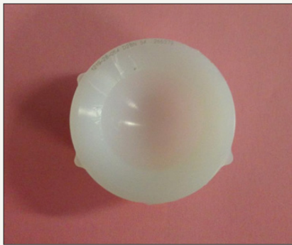
Figure 28: Dissociated Pinnacle polyethylene liner showing three of the six locking tabs have sheared off.
