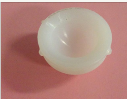
Figure 29: Only three of the six derotation locking tabs remain.
