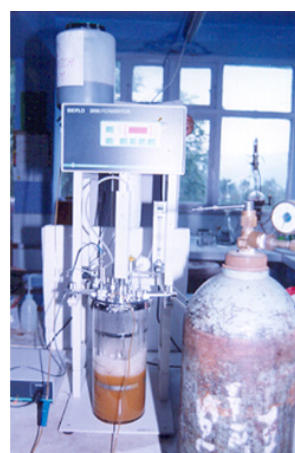
Figure 4: Production of Baker yeast from apple pomace using fed batch culture system in Bio flow 2000 fermenter.
