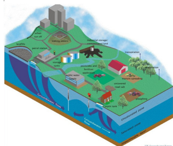
Figure 3: Water flow mechanism in river catchment area and source of pollution [20].
