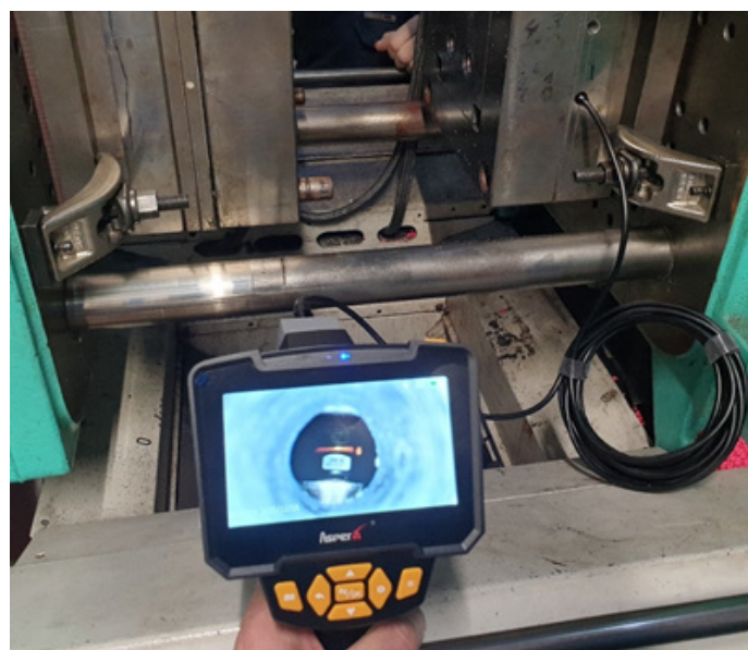
Figure 4: Monitoring the hot runner inside the mould by means of an optical sensor.
