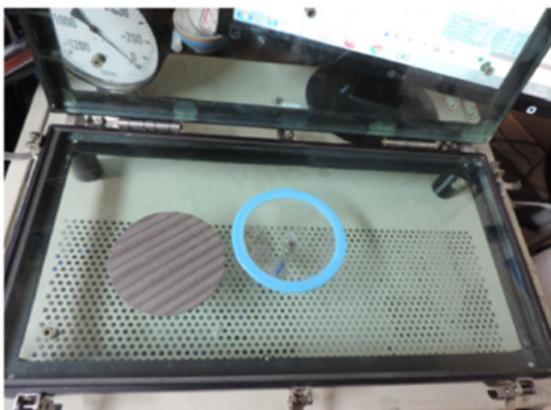
**Figure 2:** U-shaped ring seal together with a test specimen on the measuring device.
