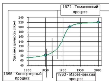
**Figure 1:** Dependence of steel specific strength on time.
