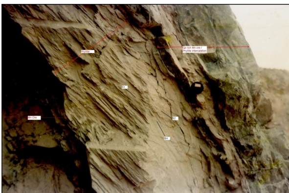
Figure 7: Traces of shear planes (SH) within phyllite, hosting shear parallel manganese ore bands. Please note the superimposition of SH over S_1 , and also of S_2 cleavages over all the earlier planes. Loc. Bharweli Mines.
