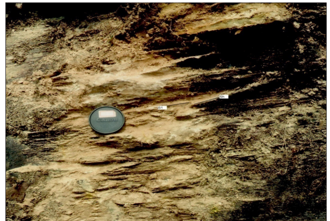
Figure 9: Angular (non co-planar) relationship between S_1 schistosity and shear planes (SH). Loc. Ukwa Mines.
