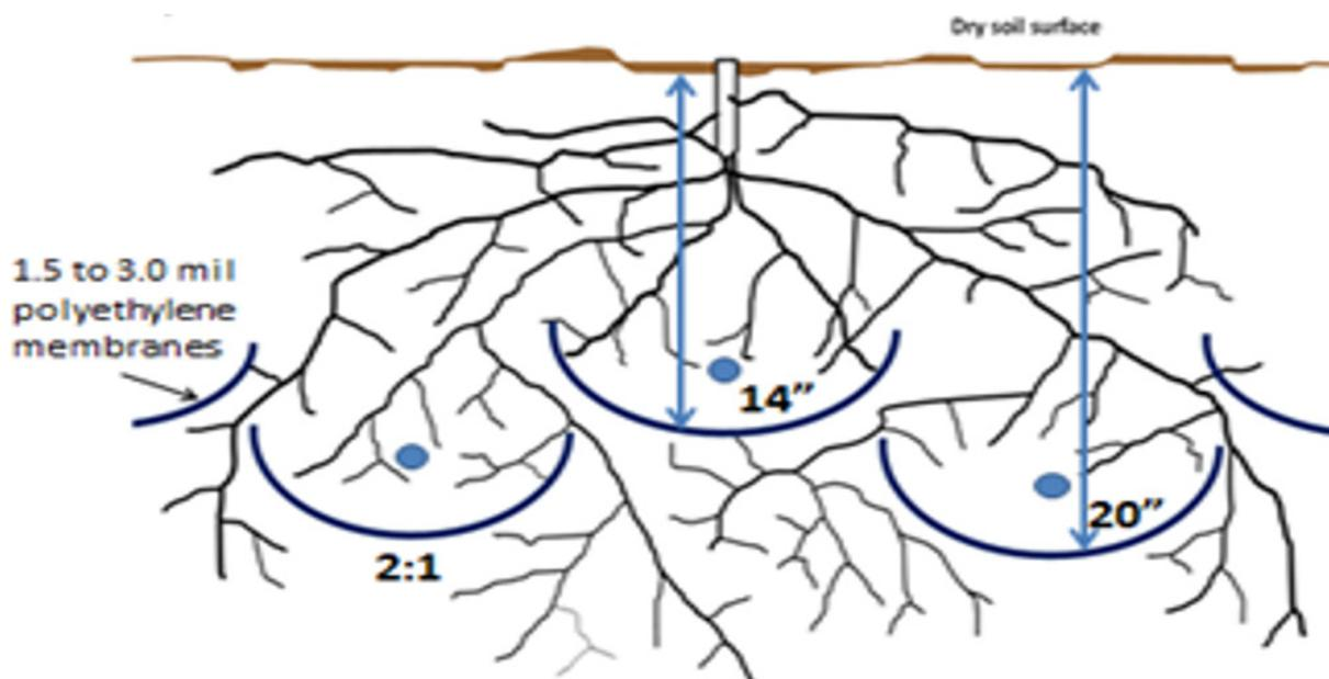
**Figure 1:** SWRT water saving membranes are contoured engineered high-density polyethylene (HDPE) films strategically spaced below plant root zone with space available for unlimited root growth and internal drainage during excess rainfall. Additions of John Deere Subsurface Drip Irrigation (SDI) pipes (.) 10cm above the SWRT water saving membranes provide best control of plant available water.
